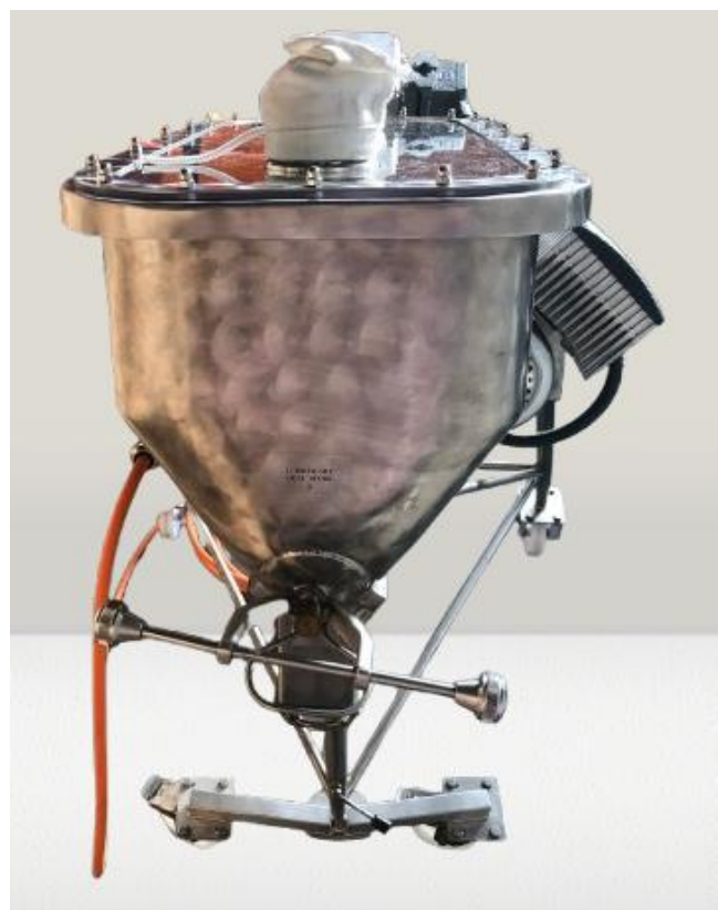
Fig. right View of product outlet and end shaft bearing to mixing screw
