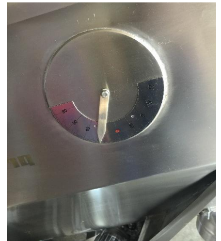
Fig. right Mechanical tilt angle indicator
