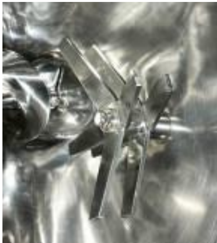
Fig. left High frequency shear head: double row blades
