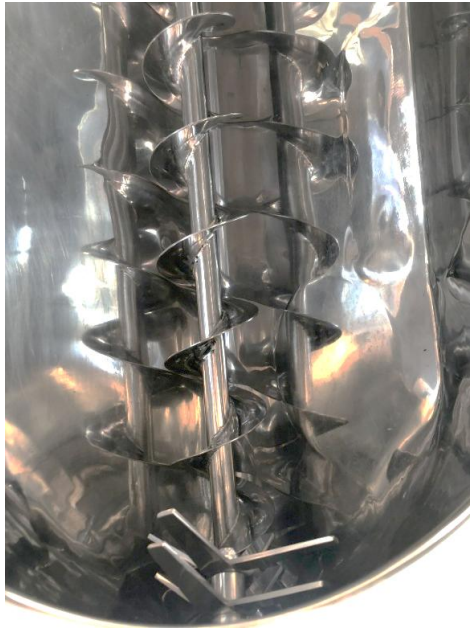
Fig. left Inside mixing hopper polished; knife head double row blades
